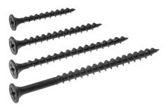
**Product description:** Type THN according to EN 14566, made of steel, specially treated, black phosphated, according to DIN 18182-2, with trumpet head, rolled tip, cross recess PH size 2 and coarse thread.
