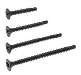
Product description: Type TMD according to EN 14566, made of steel, specially treated, black phosphated, acc. to DIN 18182-2, with trumpet head, drill tip, cross recess PH size 2.
