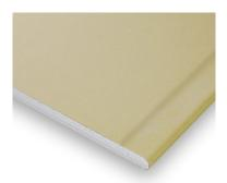
**Product description:** Gypsum plasterboard acc. to DIN EN 520, type DFH2IR, moistureresistant, made of a gypsum core with high surface hardness, dense gypsum core encased in cardboard.
