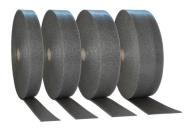
**Product description:** Tape made of Polyethylenfoam (PE), self-adhesive on one side with protective film strip. **Area of application:** For connecting lightweight partition walls or suspended ceilings to adjacent solid concrete or masonry components.
