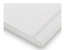
**Product description:** Gypsum plasterboard acc. to DIN EN 520, type A, made of a gypsum core encased in cardboard. **Area of application:** For installation of wall- and ceiling systems usually without fire protection requirements.
